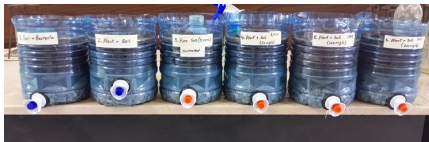
Fig. 2. Lab based Constructed wetland setup.
